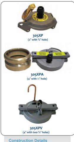
Cap body... Aluminum Cap cam levers... Aluminum (4"), brass (2") Cap gaskets... Buna-N or FKM Cable connector... Plastic Adaptor body... Brass
